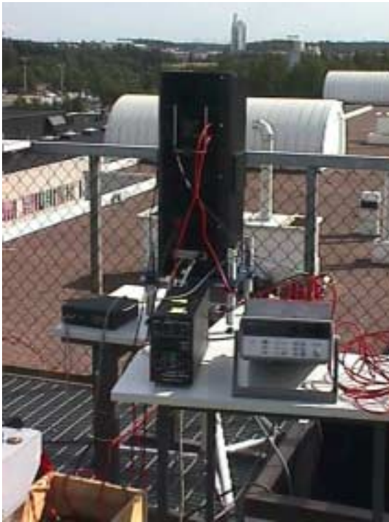
Figure 5. A photograph of the first prototype calibrator with the associated electronics for lamp control and the monitoring filter radiometers.
