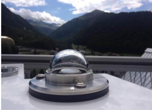
Figure 3. a) Photograph of the new Brewer diffuser b) Measured (symbols) and simulated (lines) cosine errors for the new diffuser.
