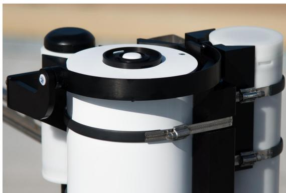
Figure 1. GUVis-3511 radiometer (center) with shadowband and GPS accessories.
