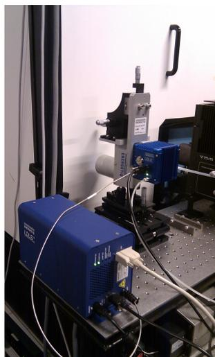
Figure 1. Laser driven light source and focusing optics on the translation stage of the spectral responsivity facility.
