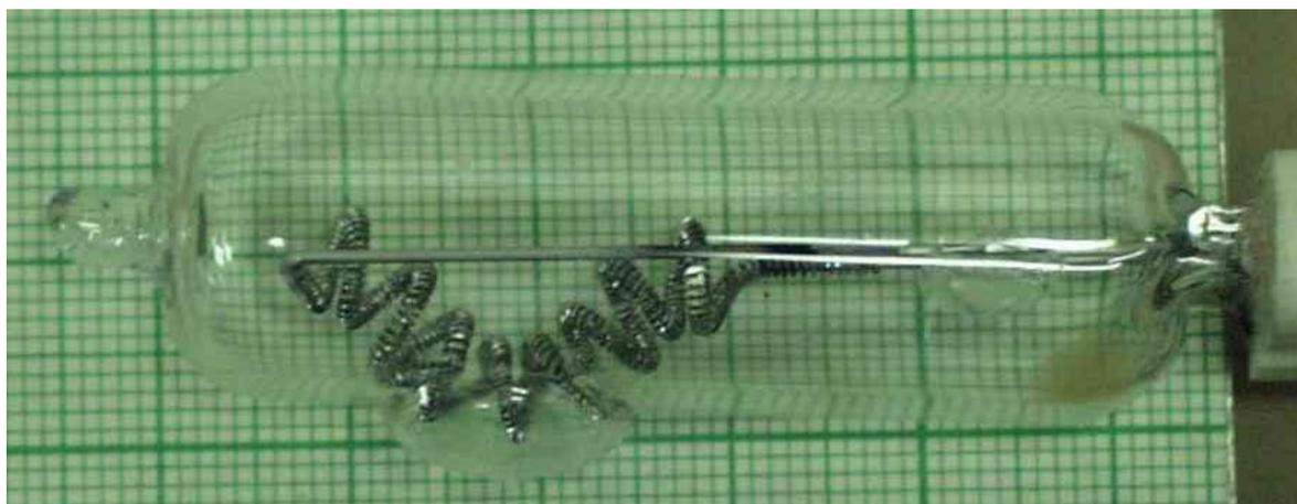
**Figure 3. Photograph showing sagging of filament and damage to lamp envelope in a horizontally operated ‘NIST’ style FEL lamp operated on a normal use cycle.**
