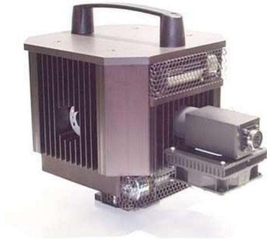
**Figure 5. Photograph of the NPL Detector Stabilised Lamp**
