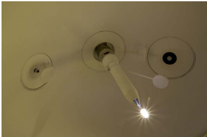
Figure 1. New custom parts of the LED luminous flux sphere.
