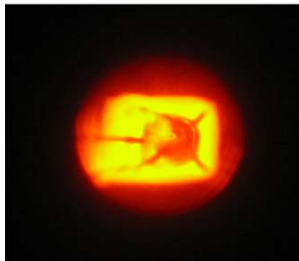
Figure 4. Image of an LED as seen by an observer in the direction of optical axis.
