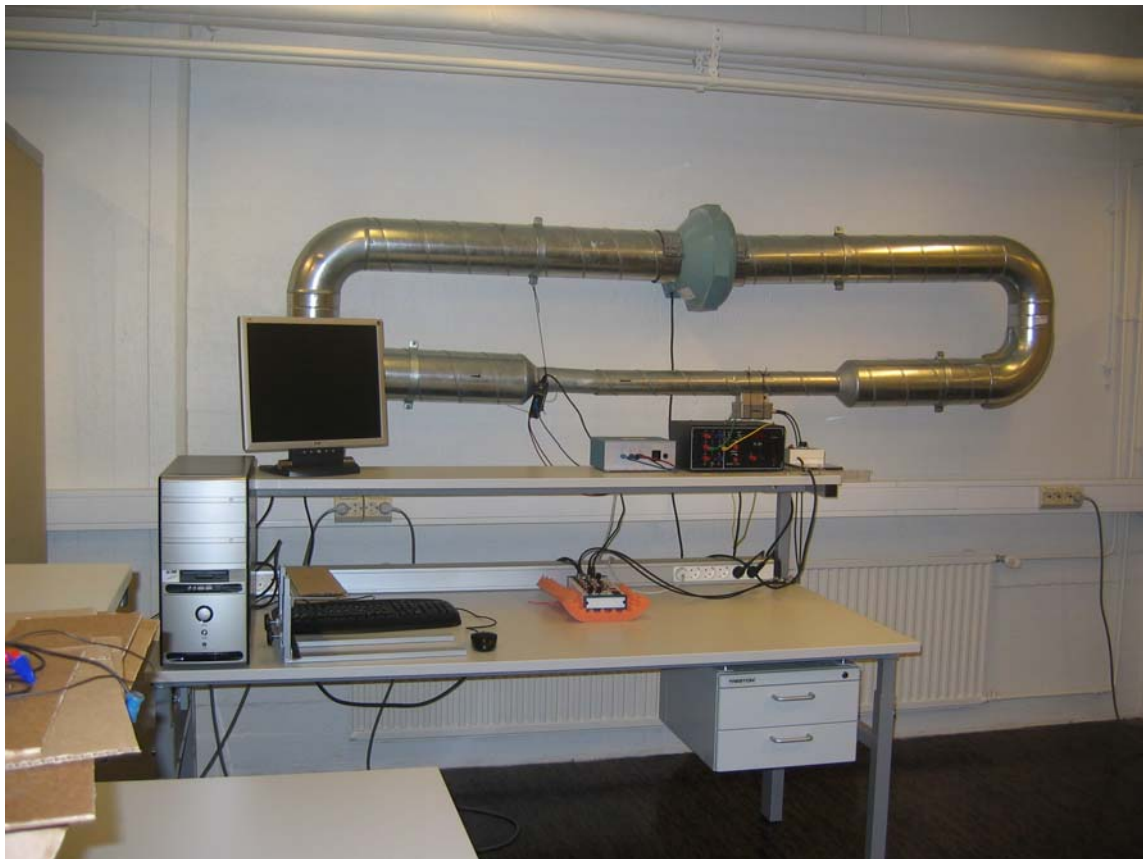
Figure 3. Experimental setup developed for teaching of measurement methods of particle velocities, cross-correlation techniques and virtual instrumentation.
