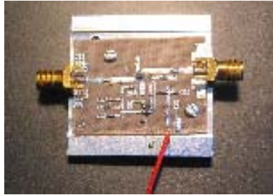
Figure 2. RF-amplifier for 5.5 GHz frequency region. The amplifier is based on a HEMT-transistor, and it is built on a circuit board made of Teflon. Surface mounted components are used to minimize non-idealities. The transmission line is a 50- \Omega microstrip.
