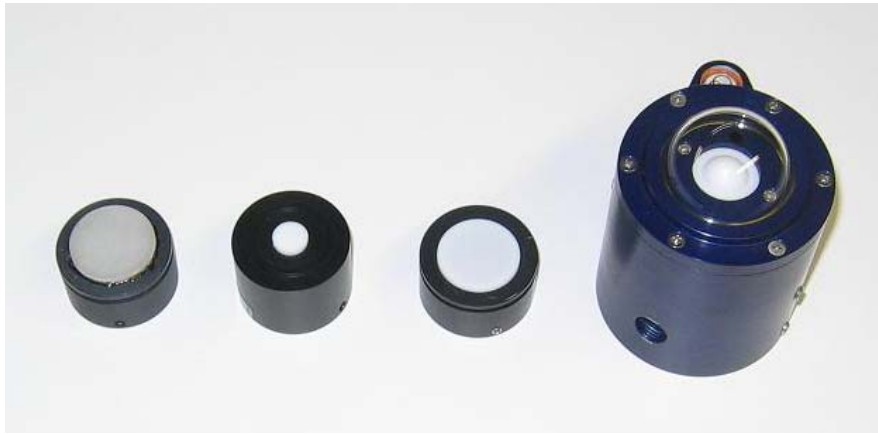
Figure 12. Studied spectroradiometer diffusers (from left to right): Bentham D3, Bentham D7, Bentham D5, and Schreder J1002-01 diffuser.
