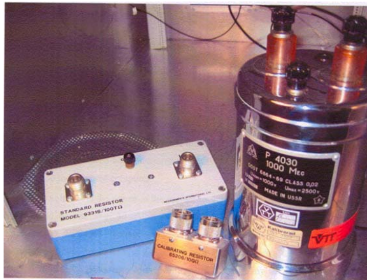
Figure 4. The 9331S-series resistor (left) and the 65206-series resistor (middle) are used in the calibrations. The P4030 1 G \Omega standard resistor (right) provides traceability for the other resistors.
